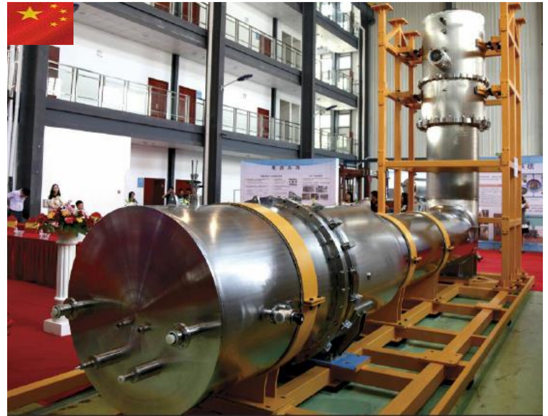
Cryogenic feedthrough for poloidal field coil #4 delivered to IO from ASIIP in October 2017, First of 31 cryostat feedthroughs to be delivered.
