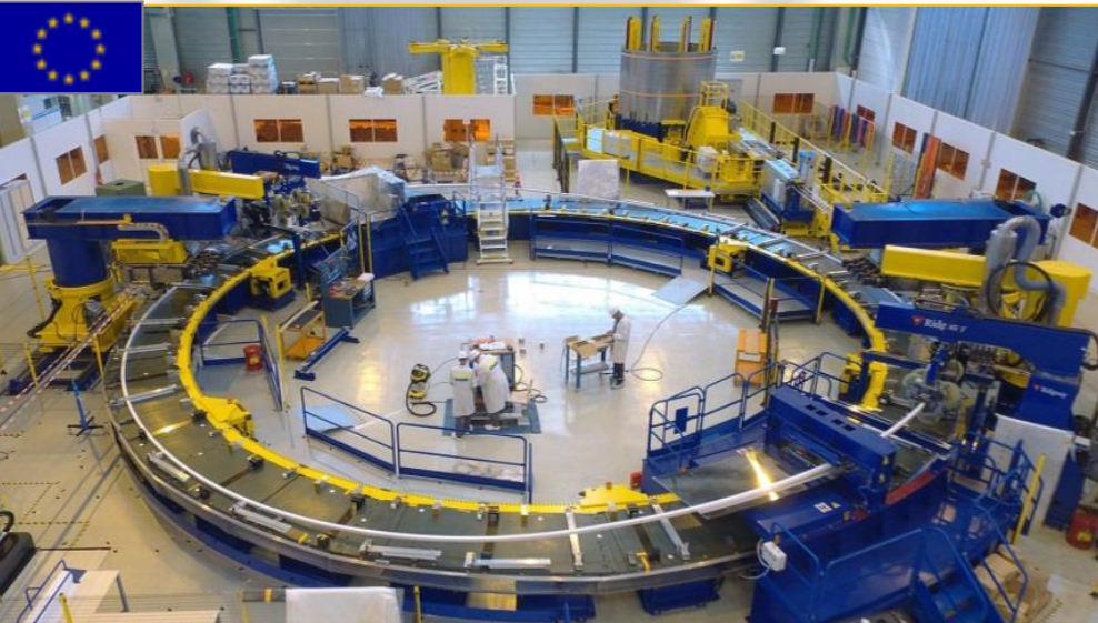
Winding of Poloidal Field Coil # 5 began in April 2017. Second pancake started by August 2017
