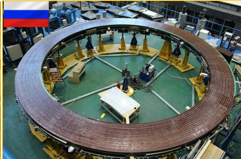
First-completed double pancake of PF1 after vacuum pressure impregnation with epoxy resin
