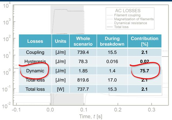
During **breakdown**, where  $\partial_t B$  peaks at **9.7** *T/s*, full saturation of strands occurs
