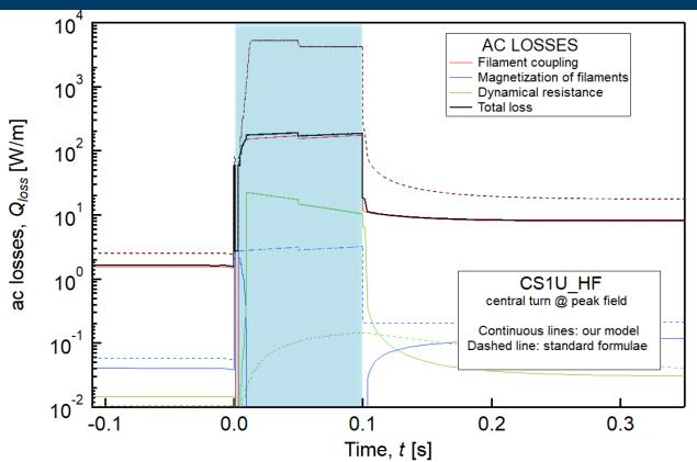
During **breakdown**, where  $\partial_t B$  peaks at **9.7** *T/s*, full saturation of strands occurs
