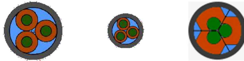
Fig.: Layout of three HTS CroCo conductor options; left: option 1, middle: option 2, right: option 3 [2].
