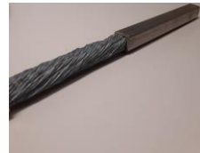
Cable-In-Conduit-Conductor cooled by supercritical helium forced-flow
