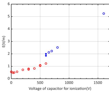
Relationship between toroidal field and voltage of ionized capacitor.
