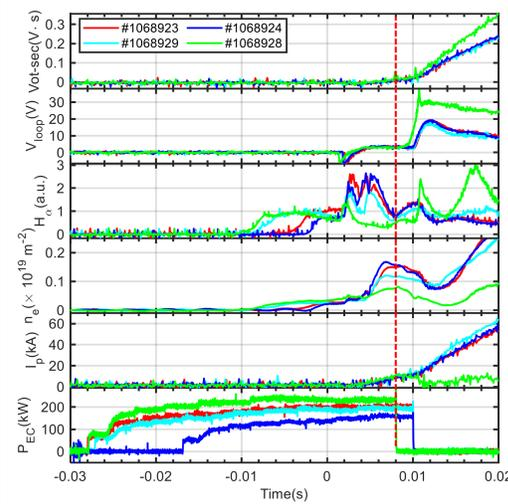
Evolution of key signals for different ECH pulse width.
