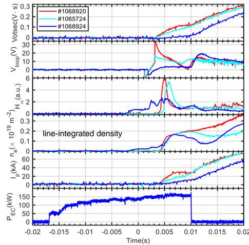
Evolution of different signals when discharging with ionization capacitor of 1600 V (red), 800 V (cyan) and 1V (blue). The last one is assisted with 300 kW ECH power while two others are pure Ohmic heating
