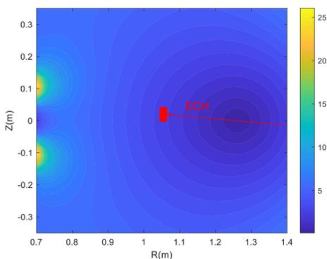
Distribution of poloidal stray field before toroidal electric field applied
