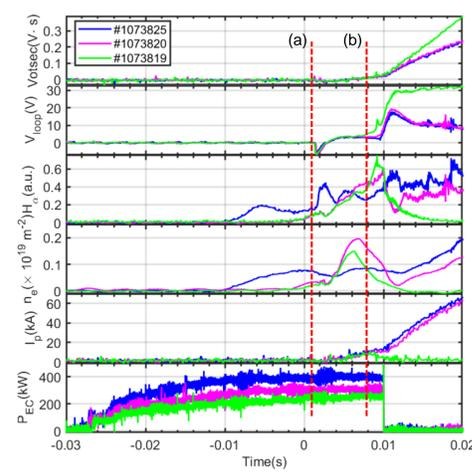
Evolution of key signals with different ECH power for assist start-up.
