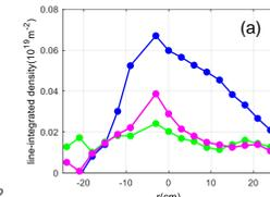
Distribution of density before toroidal field applied (t=1 ms)
