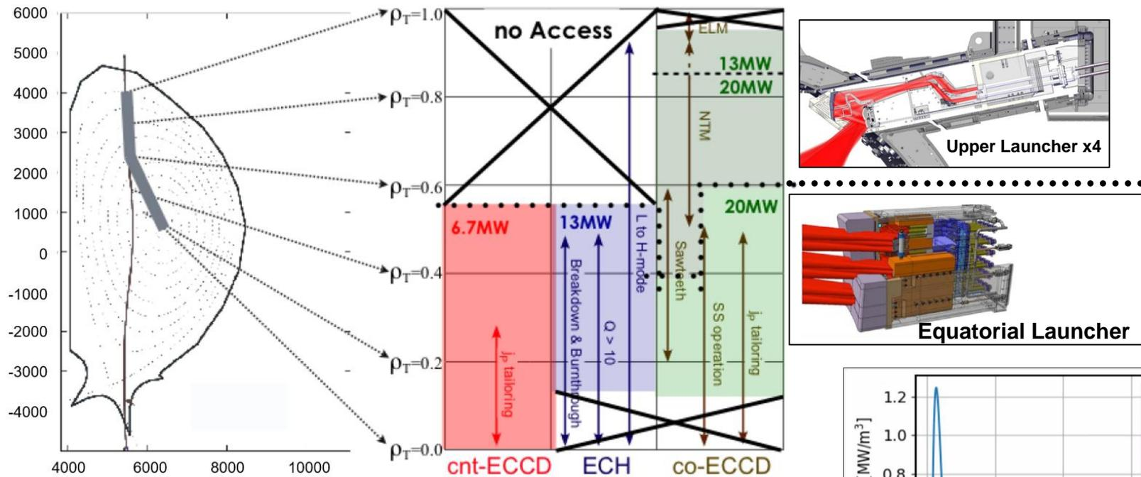
The deposition access of the EL and UL across the plasma cross section and categorized based on driving **cnt-ECCD**, **co-ECCD** or **pure heating**.
