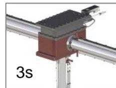
Additional Switches between upper and lower rows of the UL12 & UL13
