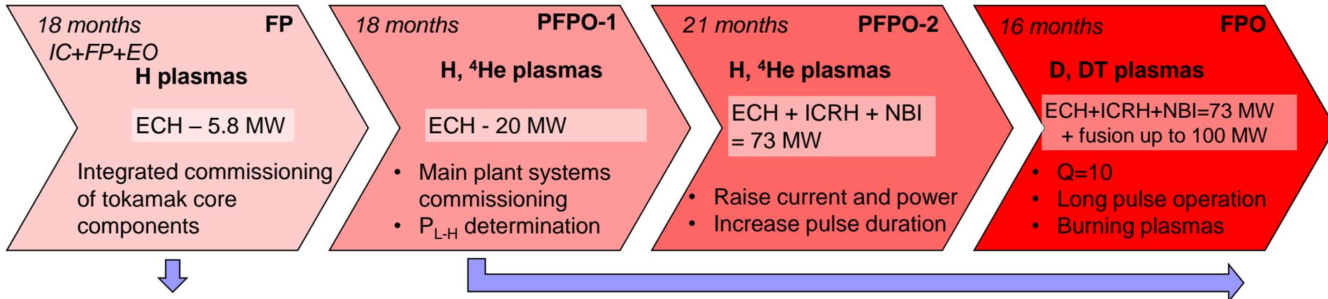
Plasma breakdown assist with ECH at 2.65T (and 5.3T in EO if needed after FP)
