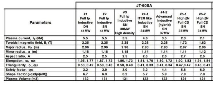
The flexibility of the ECRF system allows to consider a number of reduced B<sub>t</sub> and I<sub>p</sub> scenario besides that can be instrumental to the development of the main ones and for specific studies such as disruptions, vertical displacement events (VDEs) and run-aways build up.
