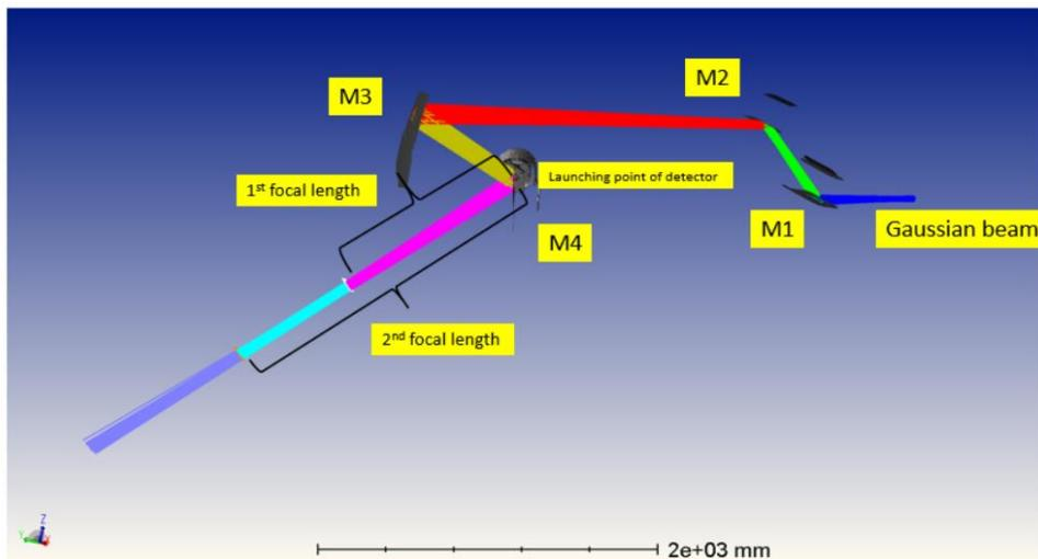
1. ZEMAX simulation reproduced the theoretical beam optics propagation in the Upper Launcher (UL).
