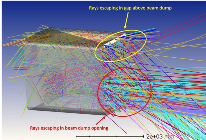
1. The gap above beam dump and opening also is checked.
