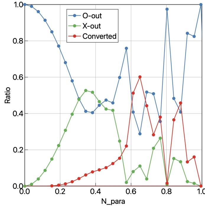
Conversion rate to EBW has maximum near the optimum injection angle ( $\sim 32 \text{ m}^{-1}$ ,  $N_{\parallel} \sim= 0.64$ ).
