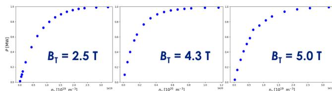
>98 % absorption in relevant densities no imminent threat of shinethrough during ordinary operation
