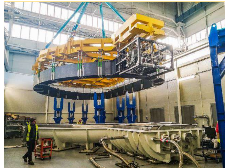
Of the 10 toroidal field coils that Europe is procuring (out of a total 19, three were recently delivered to the ITER site, TF#9 in April; TF#11 in September and TF#5 in December.
