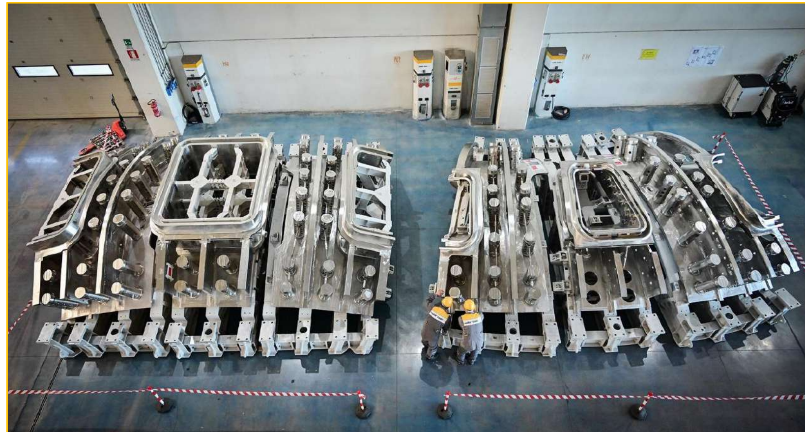
Five vacuum vessel sectors are under fabrication in Italy. Completion rates range from 66% to 89%.
