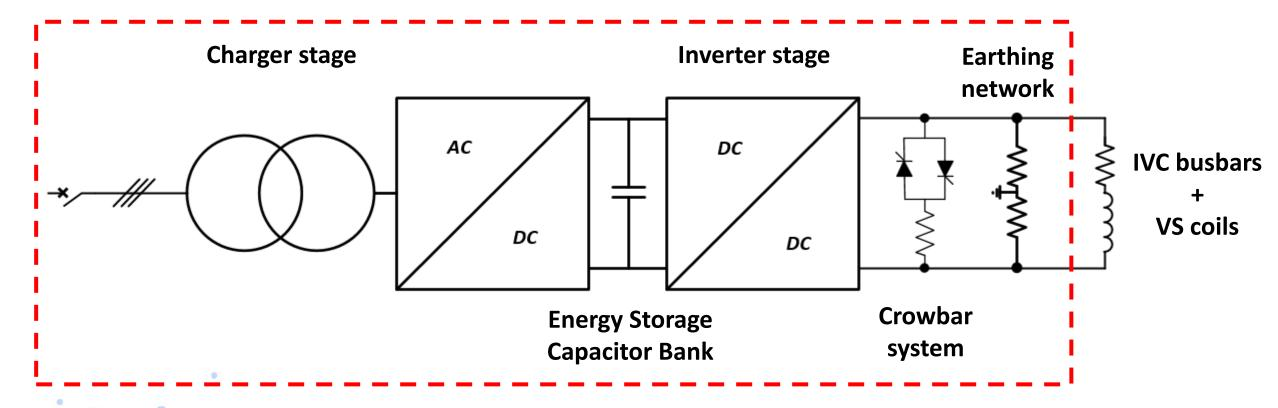
\* Safety ground switches and others protections are not represented, with the exception of Crowbar system and Earthing network.
